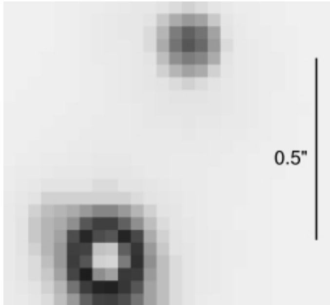
Figure 6. Reconstructed K' -image of T Tau taken with the 3D and ALFA instruments. The FWHM is 0''.14 , a Strehl number cannot be calculated because the total flux cannot be measured from this 1'' \times 1'' field of view. Spectra have been extracted on the central 2 \times 2 pixels of each PSF. The separation of the two components of the T Tau system is 0''.69
