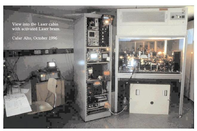
The hierarchy of oscillation frequency selection in the dye laser starts with a three-plate birefringent filter. This filter is followed by two electronically controlled etalons with progressively higher resolution. For frequency fine tuning the cavity length of the ring laser can be continuously changed by rotating a single galvo-driven Brewster plate.
